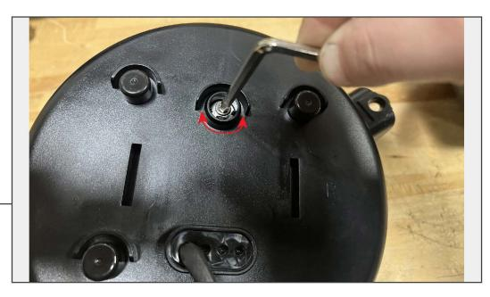
Follow the vehicle manufacturers recommendation for adjusting/aligning the headlights. Use the Allen/Phillips screws on the back of the headlight bracket to adjust the light as needed. Plug in the electronic vertical headlight adjuster if applicable. Once the lights are adjusted, follow Steps 1-4 in reverse order to complete the installation.
