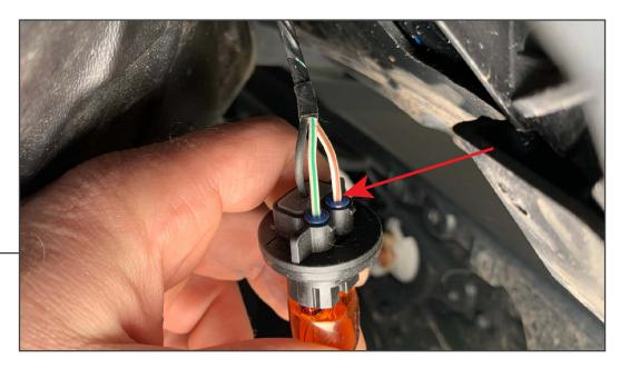
Turn the running light socket counter clock-wise and remove it from the housing. Using a test light, turn on the running lights and test for 12v+ power at the plug. On this vehicle the white/brown wire is the DRL wire. Connect the DRL wire lead to the white/brown wire. Run the spade end of the wire to the headlight bucket.
