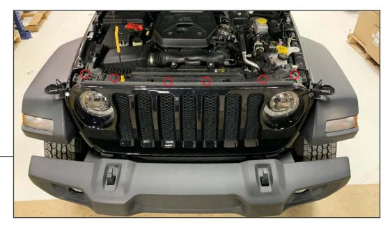
Raise and support the hood to access the (6) push clips securing the grille to the vehicle. Remove the clips and then firmly pull the grille away from the vehicle.
