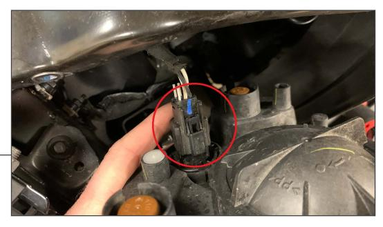
Pull the headlight away from the vehicle to access the wiring connection. Depress the connectors locking tab and pull the connector away from the light.
