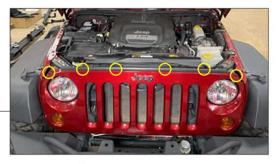
Open the hood of the vehicle. Remove (6) plastic push clips from the top of the grille.
