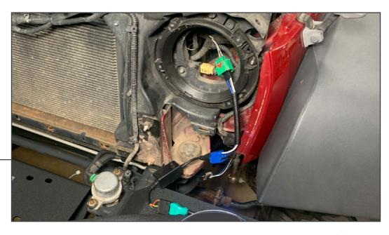
Plug the new headlight harness into the original vehicle headlight connector. Route the (2) DRL wires towards the grille mounted turn signal/parking lamp. Splice the (2) wire leads into the vehicle turn signal/parking lamp following the diagram below.
