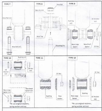
To ensure correct fitment of small mounting parts reference type number on
