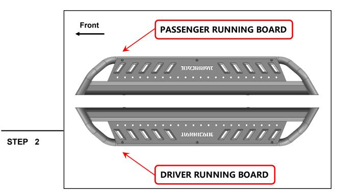
Identify each running board by identifier on the front. Notice: "D" for Driver/Left Side; "P" for Passenger/Right Side.
