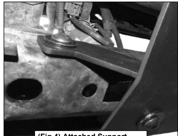
(Fig 4) Attached Support Bracket for 07-17 JK Models
