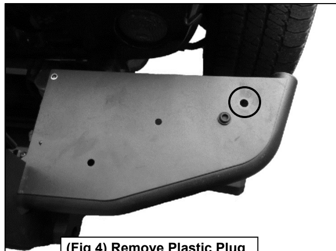
(Fig 4) Remove Plastic Plug for Push Bar installation
