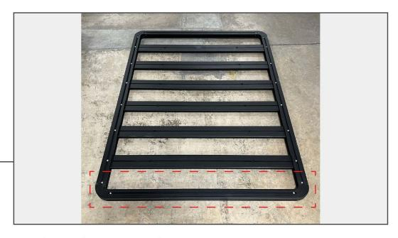
Install the rear section of the roof rack assembly following the assembly procedure in Step 2.
