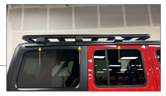
With assistance, lift the roof rack assembly onto the vehicle hardtop. Ensure all (6) mounting brackets are under the hardtop lip.
