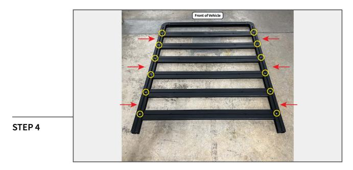
Using (6) M8 raised threaded inserts, fit the inserts into the vertical outer bars. The indicated location in the diagram above is recommended [RED].
