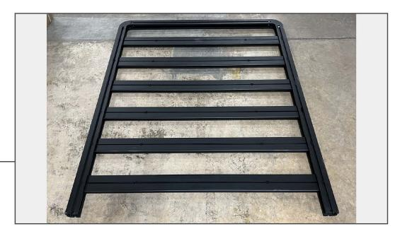
Insert the (6) cross bars into the roof rack. Do not secure into place at this time.
