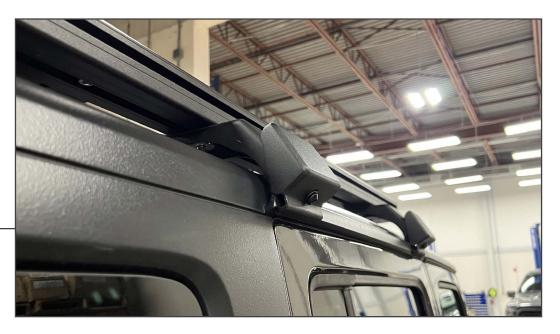
With assistance, lift the roof rack assembly onto the vehicle hardtop. Ensure all (4) mounting brackets are under the hardtop lip.
