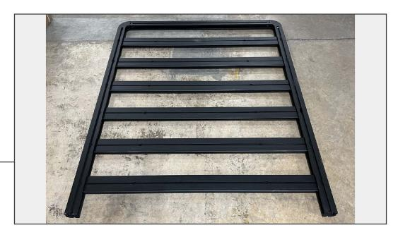
Insert the (6) cross bars into the roof rack. Do not secure into place at this time.
