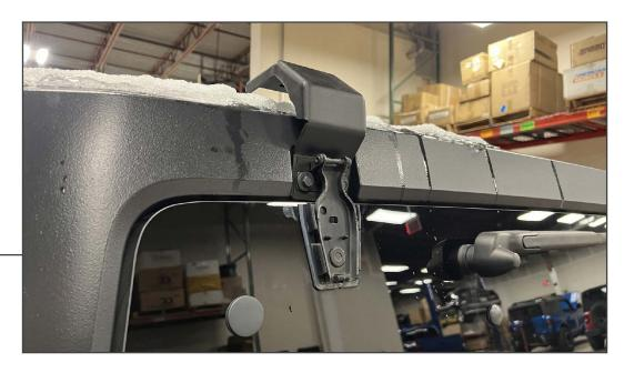
Fit (1) rear bracket between the hardtop and the glass hinge assembly. Secure the glass hinge to the vehicle reusing the original (2) 10mm bolts. With one bracket fully installed, repeat steps 6-7 for the remaining vehicle bracket.
