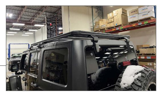
Center the roof rack to the vehicle hardtop. Then, evenly secure all hardware securing the roof rack to the brackets. Use the included (4) M8 eyelets and (4) flat threaded inserts to utilize as additional mounting points.
