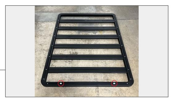
Fit (2) M8 raised threaded inserts into the rear horizontal bar, then add the corner panels and secure to the roof rack assembly following the same procedure as step 2.
