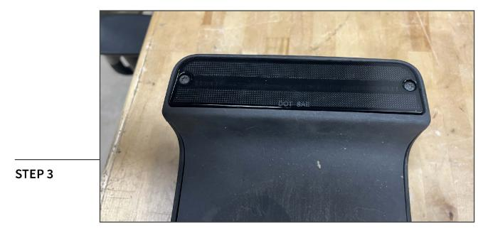
Plug the tail light into the vehicle harness, and secure the assembly to the tire carrier light housing using the original (2) T-20 Torx screws.
