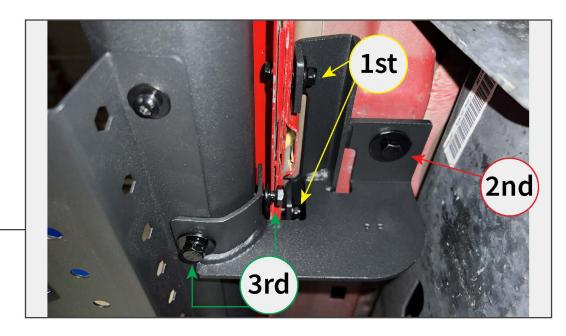
Adjust the running boards and bracket for the desired fit to the vehicle. Tighten all hardware following the diagram above.
