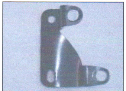
(T) Bow Assembly Brackets (Pass & Dvr)
