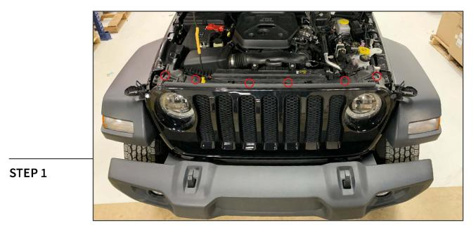
Raise and support the hood to access the (6) push clips securing the grille to the vehicle. Remove the clips and then firmly pull the grille away from the vehicle.
