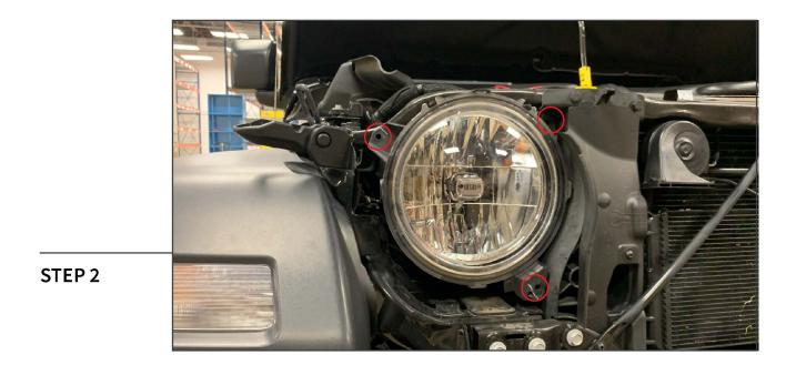
Using a 10mm socket, remove the (3) bolts securing the headlight to the vehicle.
