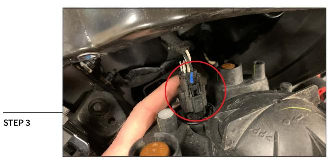
Pull the headlight away from the vehicle to access the wiring connection. Depress the connectors locking tab and pull the connector away from the light.
