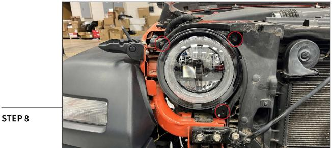
Install the LED headlight onto the vehicle using original (3) 10mm bolts. Tighten evenly until secure.
