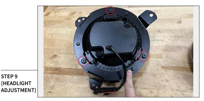
Headlight Adjustment: Tighten/loosen the (3) bolts to adjust the headlight vertically and horizontally.
