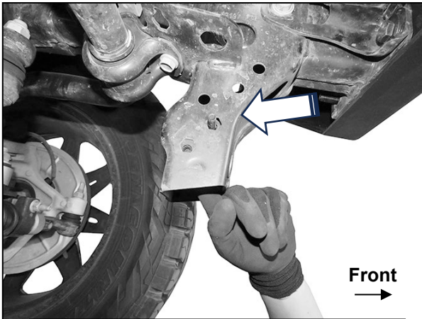
(Fig 5) For JL and JT models, insert (1) 10mm Bolt Plate into the bottom of the frame and out the hole as pictured
