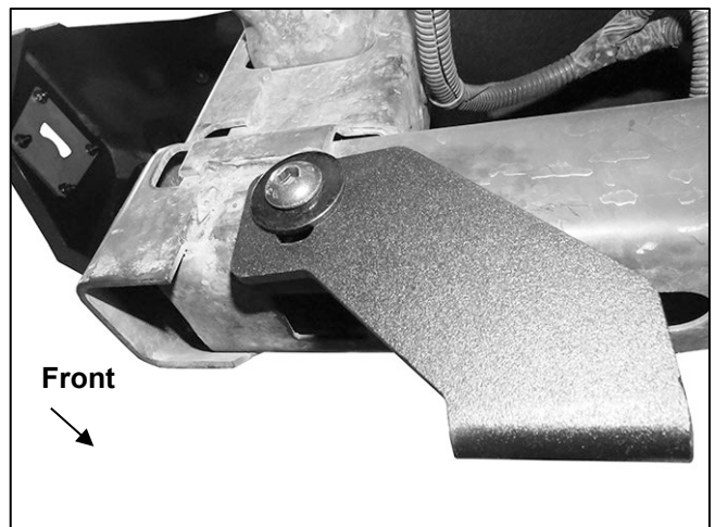
(Fig 4) JK models only, driver/left Skid Plate Bracket installed
