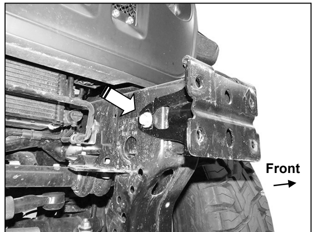
(Fig 9) JL/JT Models: Remove the inner bumper supports from the inside of the frame (arrow)
