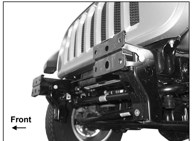
(Fig 4) Front Bumper and splash guard removed from 2018-on JL model pictured
