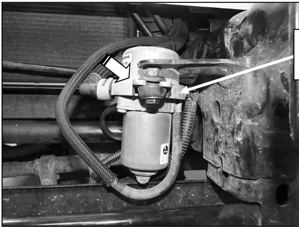
(Fig 6) JK Models equipped with vacuum servo: Use the included hardware to relocate servo to bottom of bracket (arrow)
