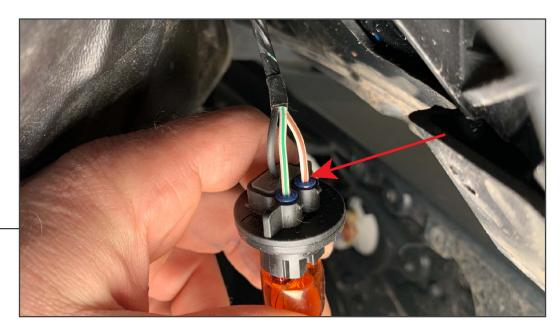
Turn the fender light socket counter clock-wise and remove it from the housing. Splice (1) wire lead into the parking lamp circuit using the included scotchlok connector. Route the wire lead to the headlight bucket.
