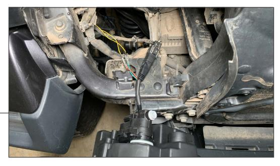
Connect the (2) wire leads to the headlight wiring. Ensure to test functionality before fully connecting the wire leads terminals together.
