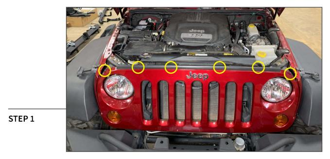
Open the hood of the vehicle. Remove (6) plastic push clips from the top of the grille.
