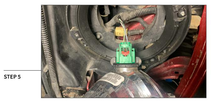
Un-plug the headlight from the vehicle. Slide the red locking tab towards the back of the connector, then press in the green plastic tab to dislodge the electrical connector from the headlight.
