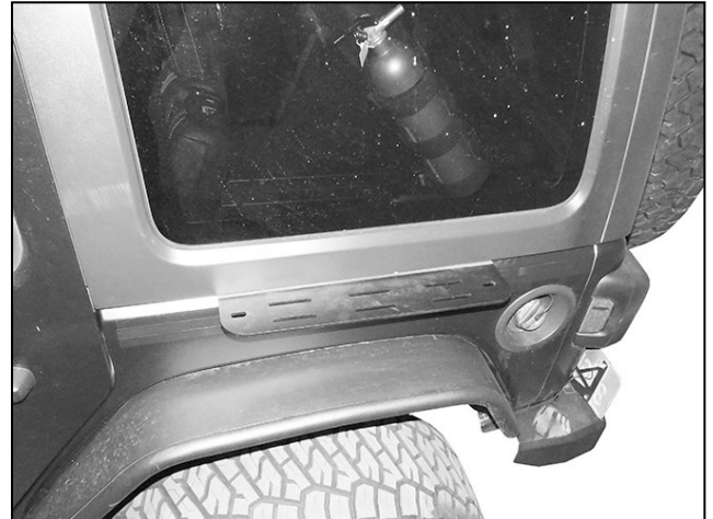
(Fig 6) Reinstall top with Bracket between top and body
