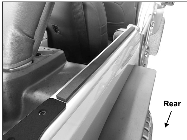
(Fig 3) Passenger/right Top and Corner Seal installed
