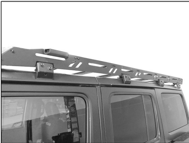
(Fig 18) Align and adjust Standoff Brackets on Rack to center Rack on roof
