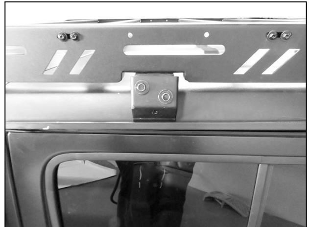
(Fig 22) Attach Center Bracket Clamp Cover to driver/left #2 & #3 Inner Mounting Brackets (driver/left #3 Bracket pictured)
