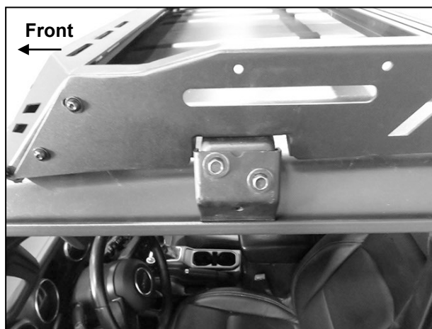
(Fig 20) Attach Front Bracket Clamp Cover to driver/left front Inner Mounting Bracket
