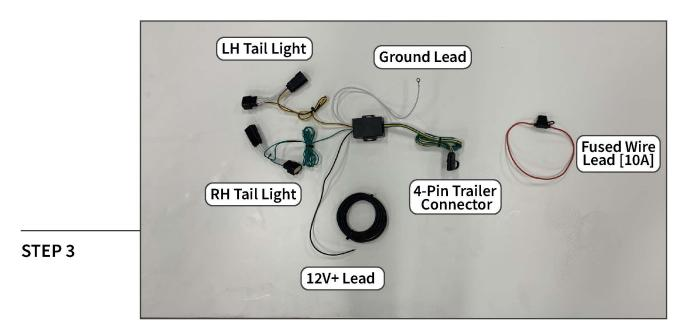
Lay out and identify each section of the wiring harness assembly.
