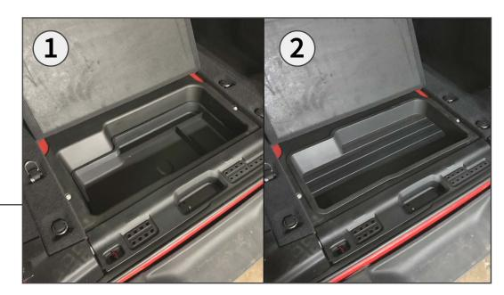
Lift the vehicle cargo area carpet to reveal the storage area. Remove all contents from the storage area.
