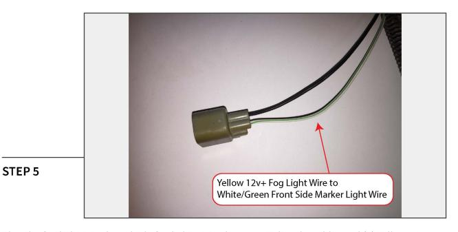
Plug the fog light into the vehicle fog light wiring harness. Splice the additional (1) Yellow wire lead to the vehicle parking light wiring in the fender flare (White/Green 12v+ wire).
