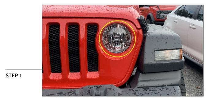
Clean the headlight buckets of the vehicle grille using exterior detailer and a microfiber cloth.
