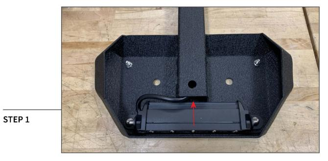
Turn the hitch step upside down, and route the wiring harness through the hitch square tube. Adjust the light bar as necessary for additional clearance.
