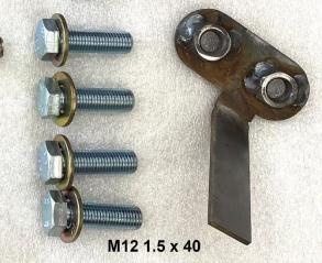
2 boits and welded nut plate to be used on the upper control arm frame bracket front two holes.
