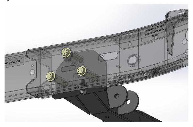
JT with no welded in sleeves. Use provided aluminum spacers as shown below.
