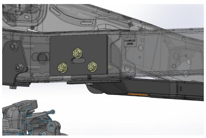
19) Next install the upper  $3^{rd}$  link bracket using the m12 bolt through the bottom of the reinfocement bracket and through the bottom of the  $3^{rd}$  link bracket. With the provided double nut plate and two m12 bolts use the opening in the outside of the frame to insert the nut plate and bolt in the front two bolts. Lastly install the 2 -  $\frac{1}{2}$  x 6" bolts through the rear of the bracket and frame into the reinforcement backet. See image below.
