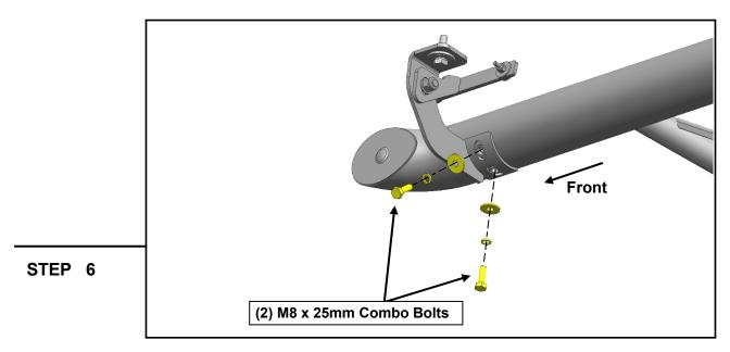
With all brackets loosely mounted to the vehicle, fit the side step onto the brackets, and loosely secure into place using (4) M8 x 25mm combo bolts.
