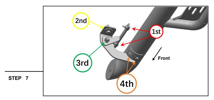
Tighten the mounting brackets to the vehicle (M6 first, then M8 / M10). Tighten the M10 bolt joining the brackets together. Adjust the side step to the desired angle, and tighten the M8 combo bolts to secure the step into place. See photo for tightening order visual.
