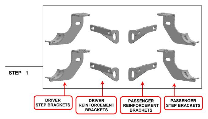
Mounting Brackets look very similar but are unique. Please Identify each mounting bracket using the engraved location identifier. Notice: The reinforcement brackets can be used in any position along the same side.
