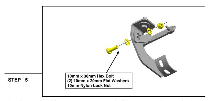
Loosely connect the (1) Passenger step bracket to the (1) Passenger reinforcement bracket using (1) M10  $\times$  30mm hex bolt, (2) M10  $\times$  20mm flat washers, and (1) M10 lock nut.
