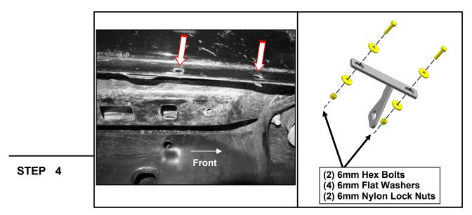
Loosely fit the Passenger Front reinforcement bracket to the inside of the vehicle pinch weld using (2) M6 x 25mm hex bolts, (4) M6 flat washers, and (2) M6 lock nuts. Do not fully tighten to allow for later adjustments. Repeat this step for all reinforcement brackets.
