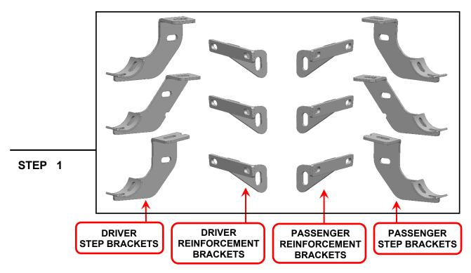
Mounting Brackets look very similar but are unique. Identify each mounting bracket using the engraved location identifier. Notice: The reinforcement brackets can be used at any position along the same side of the vehicle.
