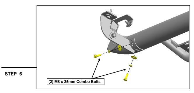
With all brackets loosely mounted to the vehicle, fit the side step onto the brackets, and loosely secure into place using (6) M8 x 25mm combo bolts.
