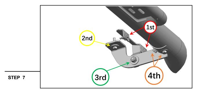
Tighten the mounting brackets to the vehicle (M6 first, then M8). Tighten the M10 bolt joining the brackets together. Adjust the side step to the desired angle, and tighten the M8 combo bolts to secure the step into place. See photo for tightening order visual.
