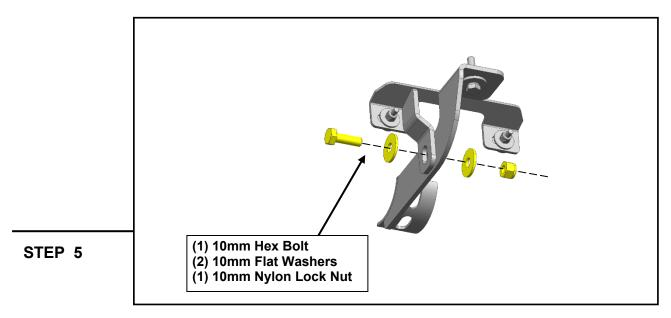
Loosely connect the (1) Passenger step bracket to the (1) Passenger reinforcement bracket using (1) M10 × 30mm hex bolt, (2) M10 flat washers, and (1) M10 nylon lock nut.
