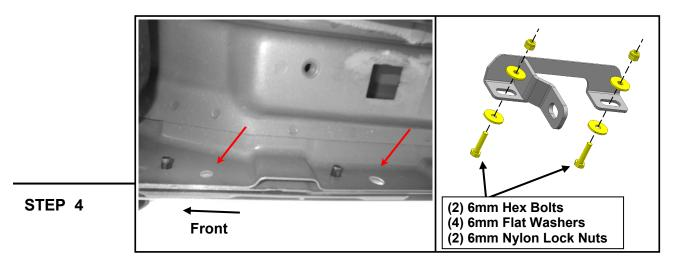
Loosely fit the Passenger Front reinforcement bracket to the inside of the vehicle pinch weld using (2) M6 x 25mm hex bolts, (4) M6 flat washers, and (2) M6 nylon lock nuts. Do not fully tighten to allow for later adjustments.
