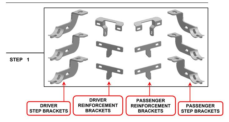
Mounting Brackets look very similar but are unique. Please identify each mounting bracket using the engraved location identifier. Notice: The center support bracket and rear support bracket per side are interchangeable.
