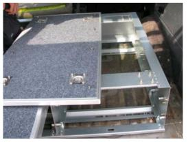
3. Adjust the position of mounting rail to fit the chair mounting point and put the screws and tighten.
