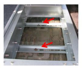
If you prefer to rise the drawer higher, you can install the Alu spacer between the bottom of the rearward mounting rib and the vehicle floor. Install a 10mm bolt and washer supplied to each side in the existing holes before Step 3.
