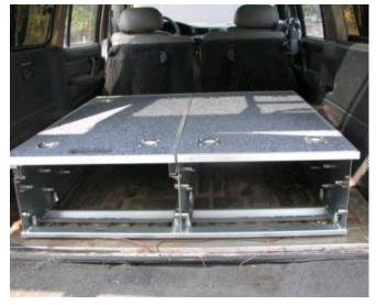
2. Loosen the screws on the hard top side (no fridge slide) to remove the hard top off.
