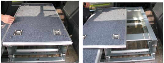
3. Adjust the position of mounting rail to fit the chair mounting point and put the screws and tighten.
