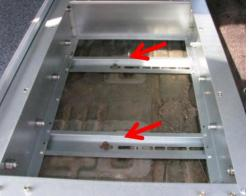
If you prefer to rise the drawer higher, you can install the Alu spacer between the bottom of the rearward mounting rib and the vehicle floor. Install a 10mm bolt and washer supplied to each side in the existing holes before Step 3.
