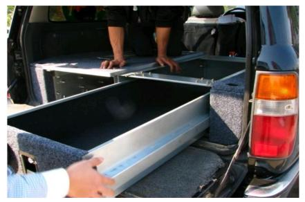
5. Put on the hard top on drawer frame and tighten the screws.
