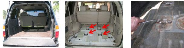
Check the distance between the chair mounting points and compare with the mounting rail at the bottom of drawer.
