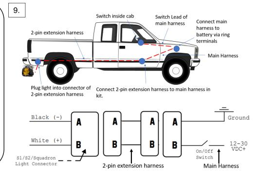
10. Now, plug in the Baja Designs S1 plug into the included wiring harness lead. Zip tie all wires so that they do not interfere with any objects and can't break free. The light should turn on when the vehicle is on and in reverse if you purchased 44-8153, otherwise if you purchased 44-8157 then the light should turn on when the vehicle is on and the toggle switch is on.
