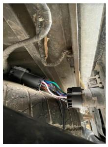
8. NOTE\* - Some vehicles have a plastic ring around the connector that prevents the included reverse harness from seating correctly. If you don't hear or feel a "click" when mating the harness to the connector, simply grab some pliers and pull the extra connector component off the stock connector. This piece is especially apparent on Ford vehicles.
