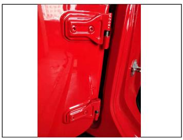
Step 5. Lift the door off the hinges and set aside.
