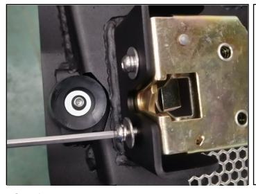
Step 1. Place the supplied M6x25mm Allen head bolt, M6 split washer and M6 mounting washer through the hole in the door and the hole in the door latch. Using a 5/32 Allen wrench tighten down slightly.
