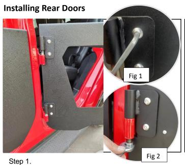
Lower the door onto the factory hinges on the vehicle. Open and close the door ensuring proper operation. Once satisfied with the function proceed to tighten down the hinge bolts using a 13 mm socket on the bolt and a 3/16" Allen head wrench on the bolts (Fig 1).
