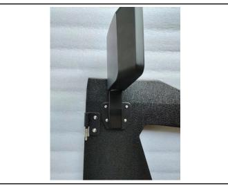
Place a supplied M6x25mm button head bolt with supplied M6 flat washer through the hole in the mirror and through the hole in the door. Place a supplied M6 flat washer and a supplied M6 split washer at the end of bolt. Start a supplied M6 hex nut at the end of bolt. Repeat step for remaining bolts. Once all bolts are installed tighten down all bolts using a 10mm socket.
