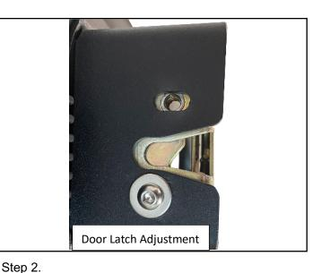
Grab door latch handle and begin to adjust the door latch forward and backward until find the proper position (this might take a few tries). Close the door to make sure there is no rattling.
