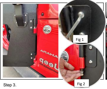
Lower the door onto the factory hinges on the vehicle. Open and close the door ensuring proper operation. Once satisfied with the function proceed to tighten down the hinge bolts using a 13 mm socket on the bolt and a 3/16" Allen head wrench on the bolts (Fig 1).
