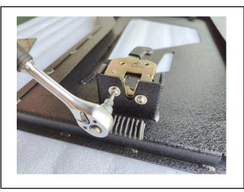
Step 1. Place the supplied M6x25mm Allen head bolt, M6 split washer and M6 mounting washer through the hole in the door and the hole in the door latch. Using a 5/32 Allen wrench tighten down slightly.
