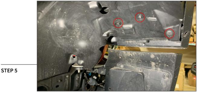
Fold back the fender liner to access the fender marker light wiring. Remove the (2) 8mm screws and (1) push clip.
