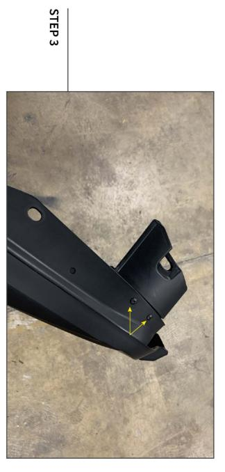
Using the supplied (2) Phillips screws per side, attach each upper grille mount to grille assembly.
