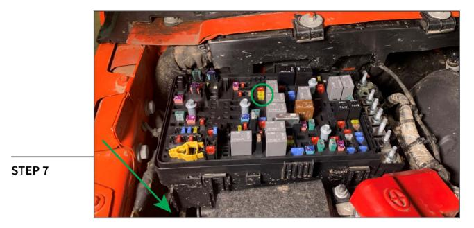
Fit the fuse tap to the RED wire harness lead, and fit into the vehicle fuse box at the indicated fuse [F58]. Neatly route the harness outwards, and then attach the ring terminal connector to the BLACK wire lead. Connect the ring terminal to the vehicle battery negative terminal.
