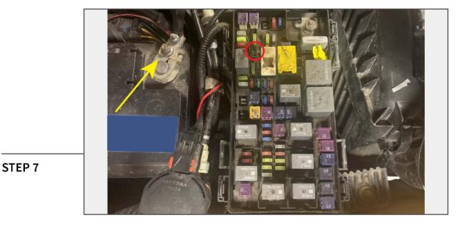
Fit the fuse tap to the RED wire harness lead, and fit into the vehicle fuse box at the indicated fuse [M9]. Neatly route the harness outwards, and then attach the ring terminal connector to the BLACK wire lead. Connect the ring terminal to the vehicle battery negative terminal.
