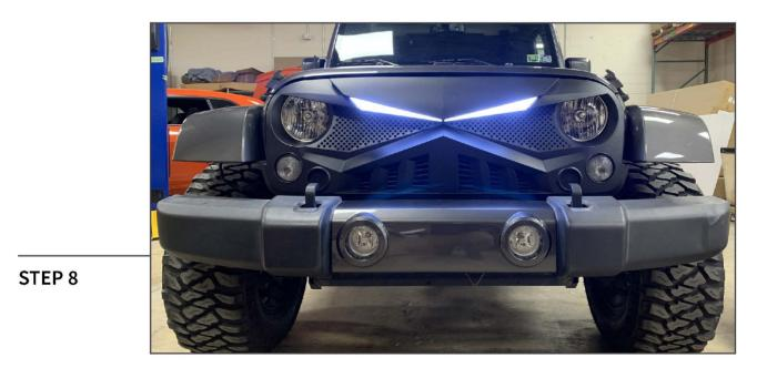
Press the grille to the vehicle, ensuring to engage all (6) lower metal retaining clips. Then, secure the top of the grille using the (6) plastic push clips. Using the attached double sided tape, adhere the weather seal to the top of the grille centered with the vehicle.
