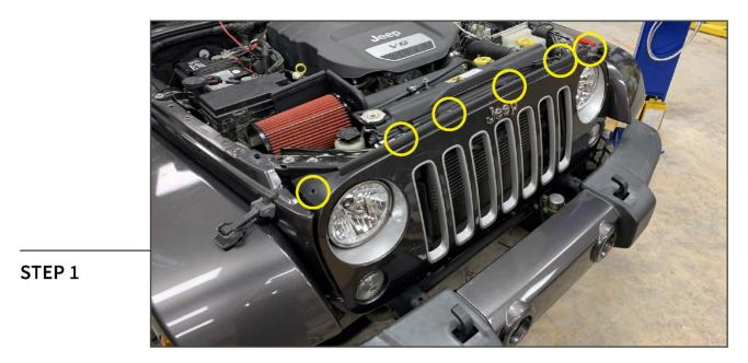
Open the vehicle hood. Remove (6) plastic push clips from the top of the grille assembly.
