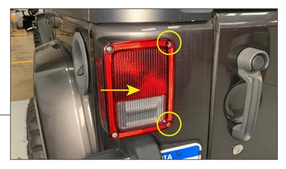
Remove the (2) inner Phillips head screws from the tail light assembly. Push the tail light towards the middle of the vehicle to dislodge the inner clips.
