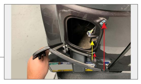
Align the alignment tab in the tail light bracket to the vehicle, then push the panel inwards to lock the outer tabs into place. Ensure the (2) bolt holes remain aligned with the vehicle. Once properly aligned, press the tail light bracket into the vehicle to adhere the tape to the vehicle body panel.
