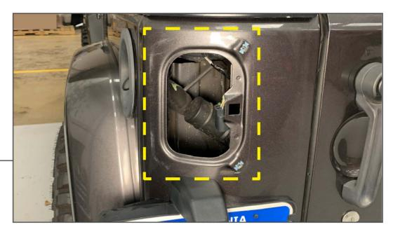
Clean the tail light mounting area of the vehicle using isopropyl alcohol and a microfiber cloth. Allow the vehicle to fully dry.
