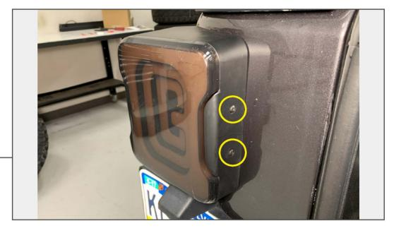
Align the tail light to the tail light bracket on the vehicle. Plug the tail light into the vehicle harness. Secure the resistor secured to the resistor bracket to the vehicle metal behind the tail light area using the (2) 'S' clips. Secure the tail light into place using (2) small Phillips screws.
