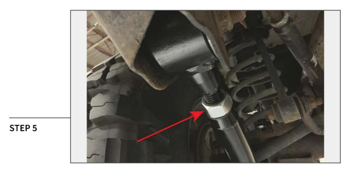
Using an adjustable wrench, tighten the jam nut to secure the control arm adjustment.
