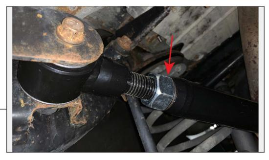
Using an adjustable wrench, tighten the jam nut to secure the control arm adjustment.
