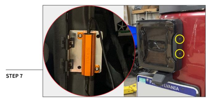
Secure the resistor to the provided resistor bracket using (2) M4 bolts and (2) M4 nuts, tighten until secure. Then, secure the resistor to the vehicle chassis using (2) "S" clips.
