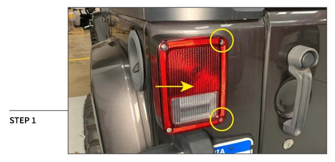
Remove the (2) inner Phillips head screws from the tail light assembly. Push the tail light towards the middle of the vehicle to dislodge the inner clips.
