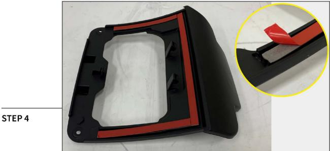
Remove the tape backing from the 3M tape attached to the tail light bracket.
