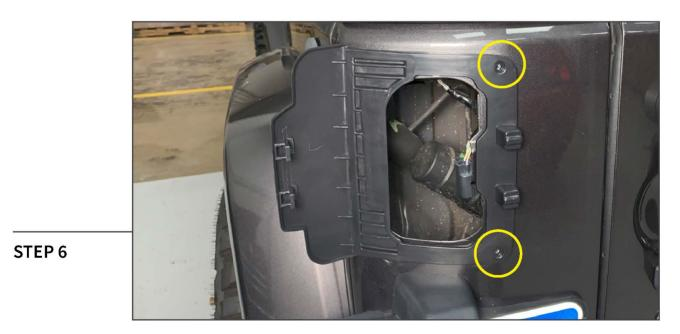
Secure the tail light bracket to the vehicle using the (2) original Phillips head tail light screws.
