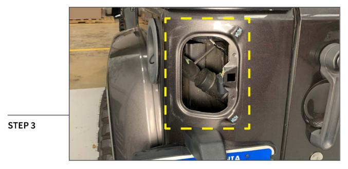
Clean the tail light mounting area of the vehicle using (1) alcohol prep pad.
