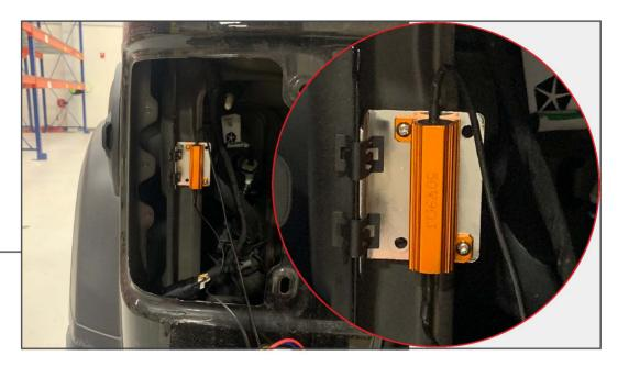
Using the provided clips, install the resistor and bracket onto the pinch weld behind the tail light.
