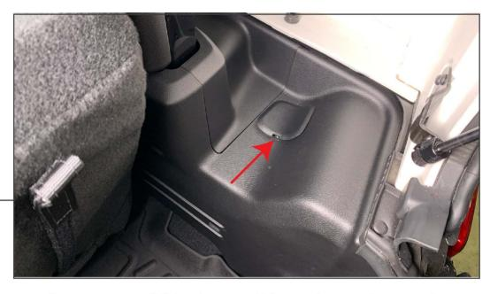
Begin by opening the tailgate to access tail light trim cover. Using a soft pry tool, remove the cover from the vehicle.
