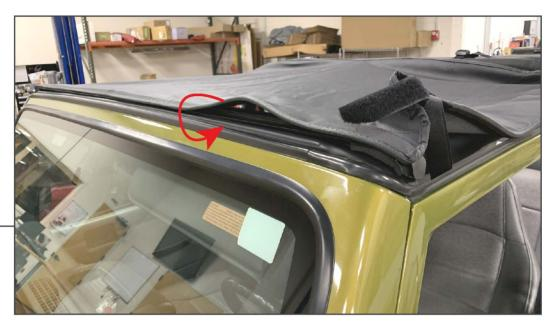
Fit the front of the top to the previously installed header panel. The plastic strip will fit into the header panel groove.
