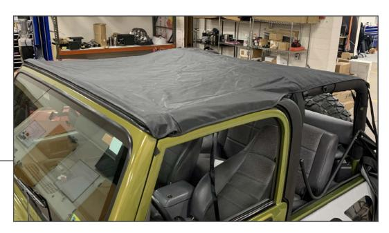
Ensure all straps are tight and secure. Secure the front corner Velcro straps together around the front of the roll bar.
