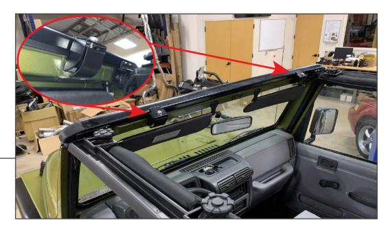
Remove the vehicle top from the vehicle. Installation of the REDROCK header panel is required for installation (SKU # J181078).
