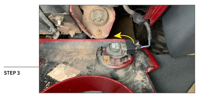
Twist the turn signal socket to remove the turn signal bulbs from the grille. Remove the grille from the vehicle.
