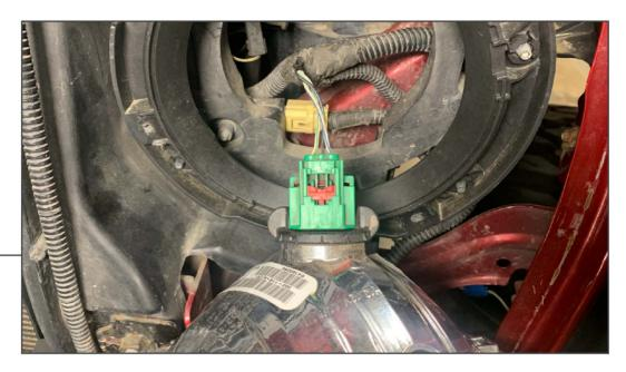
Un-plug the headlight from the vehicle. Slide the red locking tab towards the back of the connector, then press in the green plastic tab to dislodge the electrical connector from the headlight.
