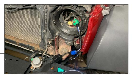
Plug the new headlight harness into the original vehicle headlight connector.
