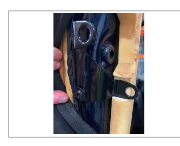
6. Locate (1) Side Bow and (2) Billet Disconnect Pin w/ Clips. Attach top section of the Side Bow to the Rear Door Surround Bracket and secure it with Billet Disconnect Pin.
