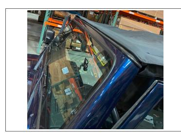
14. Insert the rear corners of the Soft Top into the rear corner belt rail.
