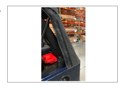
15. Start horizontal and vertical zippers on the quarter window about 4-6 inches. Insert the plastic strip on the bottom of the quarter window into the Side Belt Rail.
