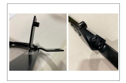
3. Orient Door Surround Assembly on the vehicle with the Brackets towards the inside of the vehicle. Line up the Threaded Nipples with the holes on the bottom of the roll bar. Secure the Door Surround Assembly to the roll bar by inserting Knobs from the top of the roll bar until it reaches the Threaded Nipples. Do not tighten at this time.
