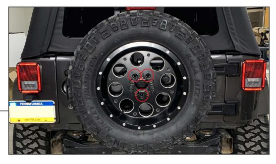
Remove the spare tire from the vehicle by removing the (3) lug nuts.
