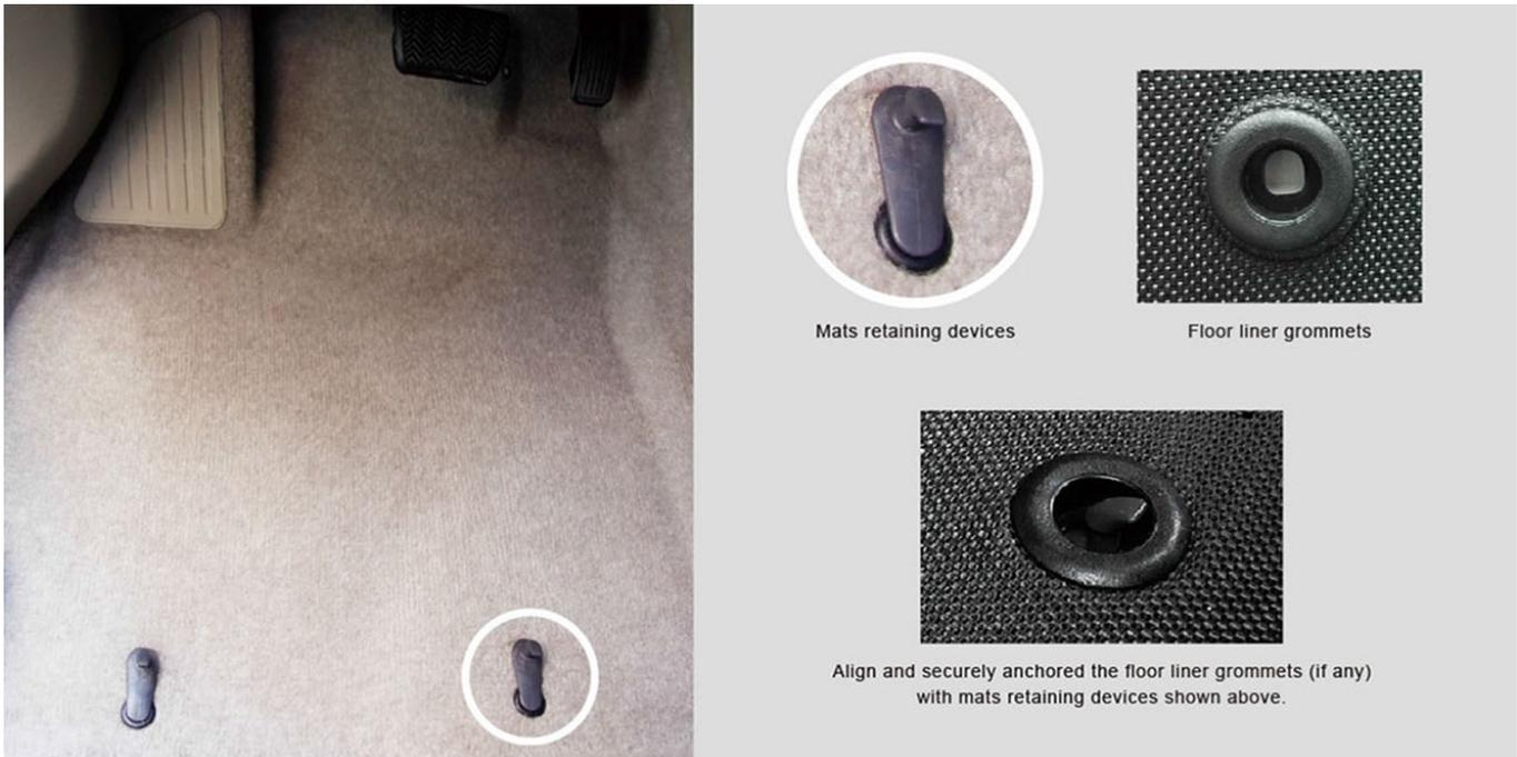
Step 4. With the engine stopped and the shift lever in P, fully depress each pedal to the floor to make sure it does not interfere with the installed floor mat.
