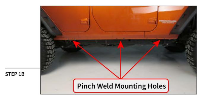
The metal clips are located directly behind each pair of pinch weld mounting holes. (4-door Wranglers only need threaded clips on the front and middle locations).
