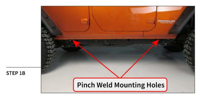
The metal clips are located directly behind each pair of pinch weld mounting holes.
