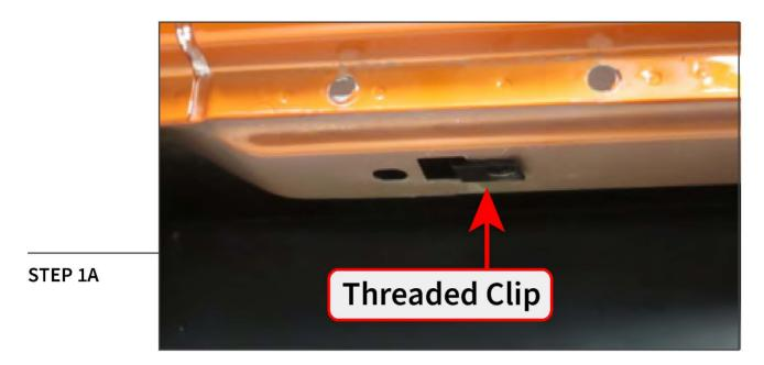
Begin by installing (2) threaded metal clips on the underside of the body.
