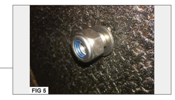
Insert (5) M10x1.50 x 25mm bolts through the drilled holes. Secure the rocker guard to the vehicle by using (5) M10 flat washers and (5) M10 lock nuts through the back-side of the rocker guard. Tighten until secure.
