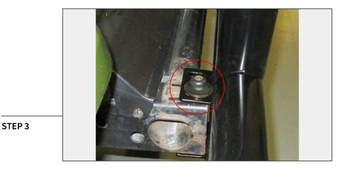
Place the front bumper over the front of the frame, with light mounts on the top. Reinstall the (2) front upper bolt through the front bumper.
