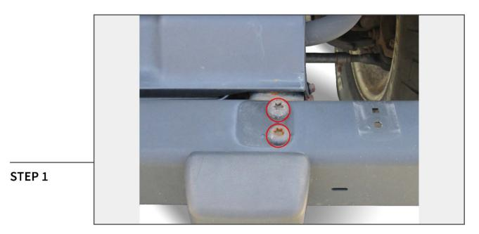
Remove the upper (4) T-55 Torx bolts from the top of the factory bumper, these bolts will be reused.
